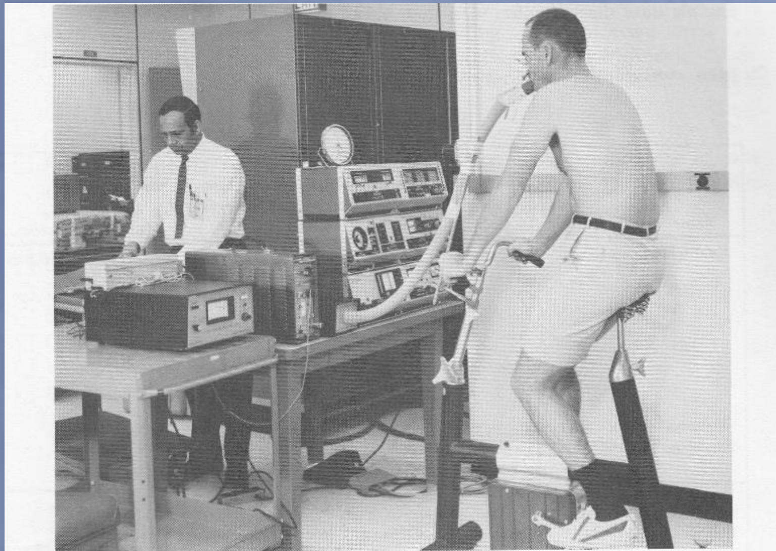
Fig. 12-2. Oxygen consumption computer. System for continuous computation and display of the amount of oxygen consumed during automatically timed 1-minute periods (by monitoring respired air) consists of a breathing mask and hose, mass flow meter, fan, oxygen polarographic sensor, heater to prevent condensation by maintaining the temperature of the sensor at 96° F., special-purpose analog computer, and two full-scale calibrators spanning the total range of applications from basal metabolism to maximal exercise. Assistant (left) collects bag samples for validation. (Courtesy NASA.)
